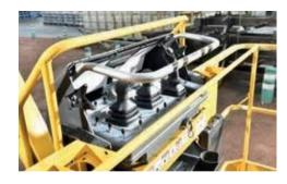
The HT28 range is equipped with a secondary guarding system: the HAULOTTE ACTIV'Shield® Bar 2.0 (standard or optional depending on models).
