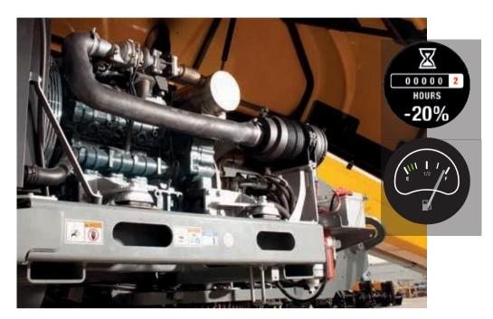
When operators are working at height, the engine often runs for no reason, resulting in the hourmeter counting hours unnecessarily. That is why the HT28 range is equipped with the innovative STOP Emission System that automatically stops and restarts the engine.
