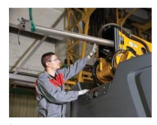
Some repairs require removal of the boom cylinder: a laborious process that often takes several days.
